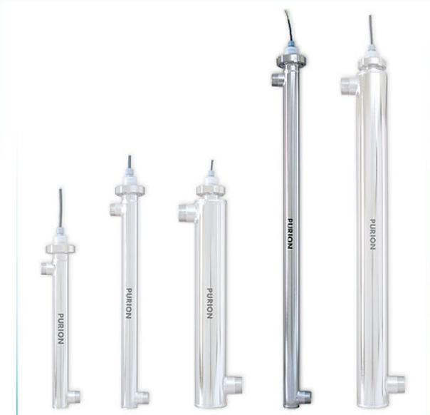
UV Plant PURION 2500 H is equipped with a polished stainless steel reactor. PURION 2500 H can be used to disinfect high temperature water especially to protect legionella. It's possible to disinfect drinking water up to a flow rate of 4.000 l/h and a transmission of at least 90% per cm.
